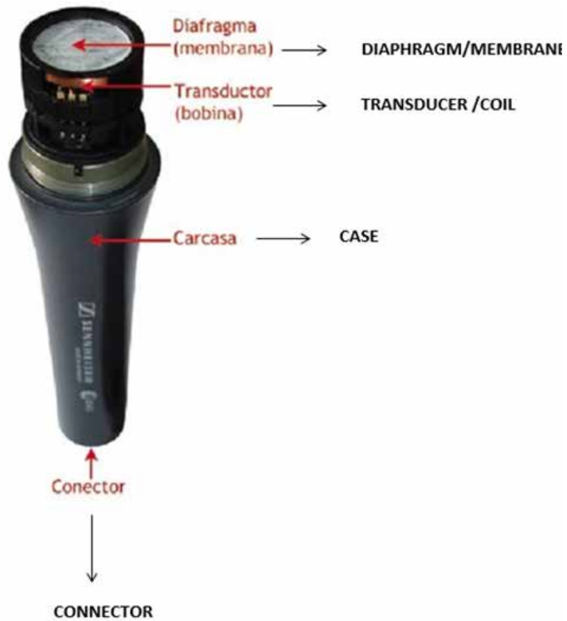
Figure 58. Microphone Internal parts
